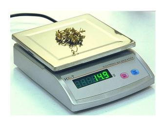
To avoid damage when transporting the balance, ensure that nothing presses on the weighing platform (if posting it, replace the screws to their original position as show in the first picture). Likewise, never leave a weight (any weight) on the weighing platform for a prolonged period.
